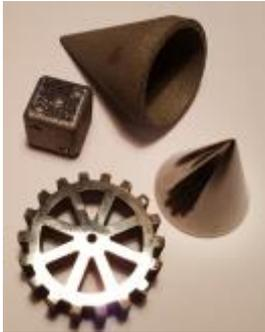
Examples of amorphous demo parts fabricated in an EOS system (Source: Exmet AB).
